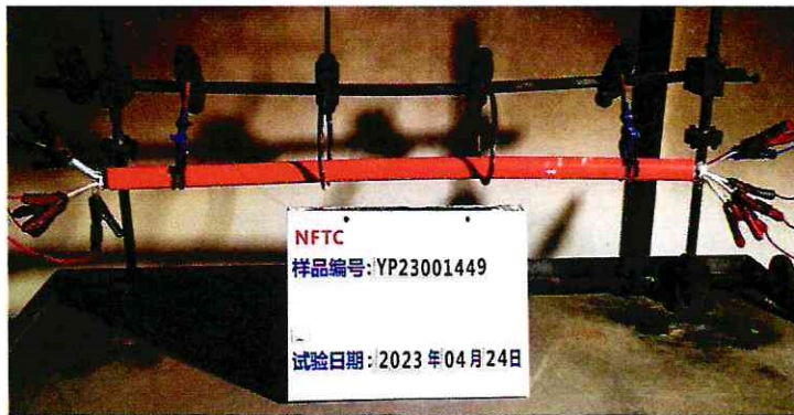
After fire test for circuit integrity
