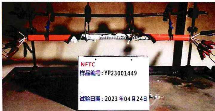
After fire test for circuit integrity
